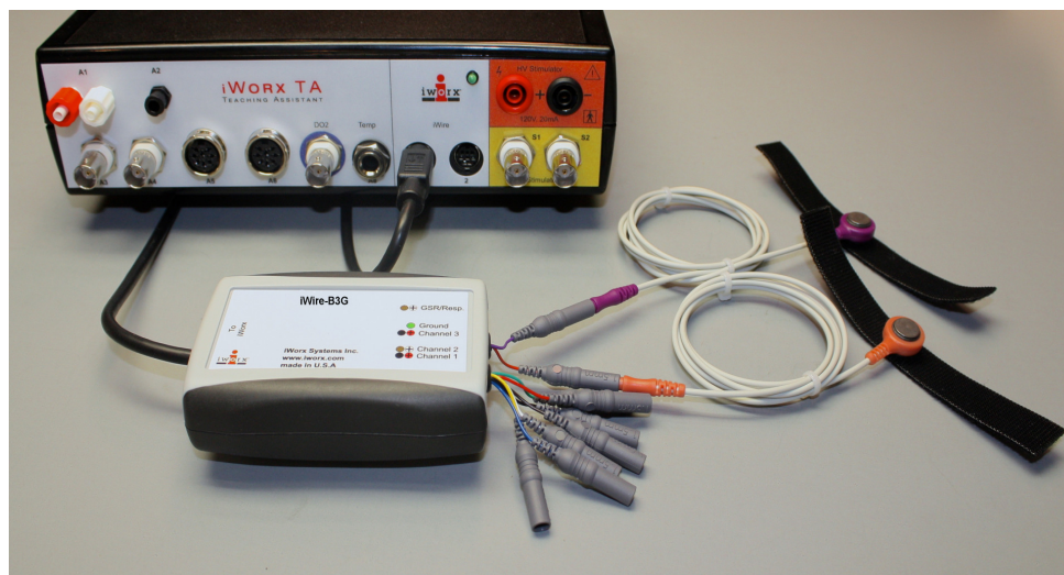
Figure HP-8-S3: The equipment needed to record GSR. The PT-104 plugs into Channel A5.
