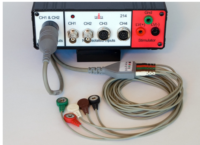
Figure HH-4-S2: The C-AAMI-504 ECG cable connected to an IWX/214.
