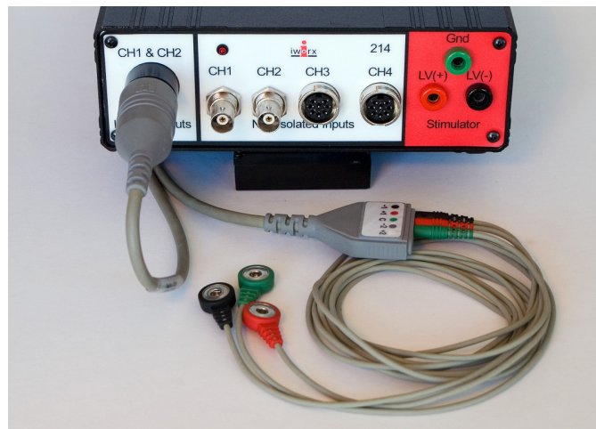
Figure HH-6-S2: The ECG cable connected to an IWX/214.
