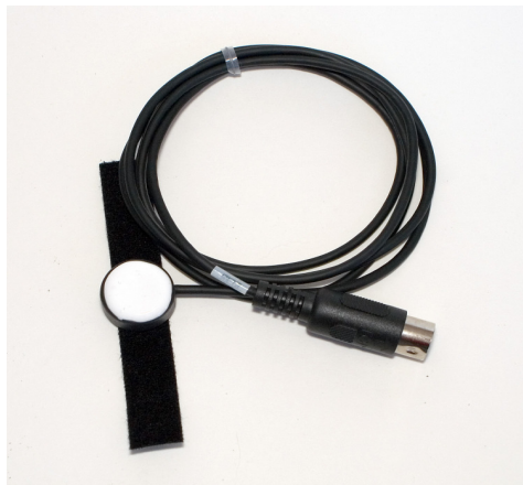
Figure HH-3-S2: The PT-104 pulse plethysmograph.
