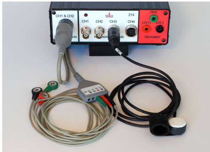
Figure HH-3-S3: The ECG cable and pulse transducer connected to an IWX/214.
