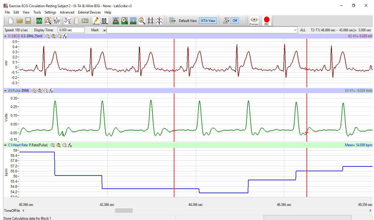
Figure HH-3-L1: ECG, pulse and heart rate displayed on the Main window.
