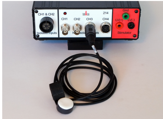
Figure HH-5-S2: The PT-104 connected to the IWX/214.
